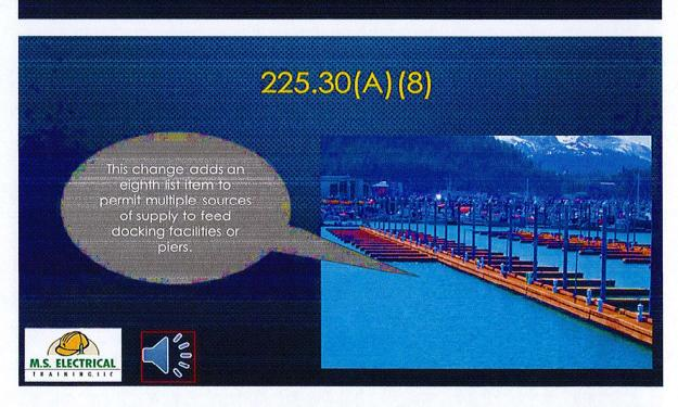
A building or other structure that is served by an outside feeder is still generally limited to only be supplied by one feeder unless another feeder is permitted by special conditions. In Section 30 (A) another special condition will now allow a new #8 – docking Facilities and Piers. Also note in Section 225.30 (B):
